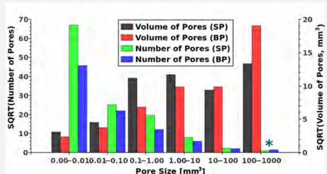
The **3D pore-size(-volume) distribution** (which has an influence on strength, permeability, density, thermal insulation, etc.) can be determined and visualized with CT on a laboratory X-ray diffractometer.
