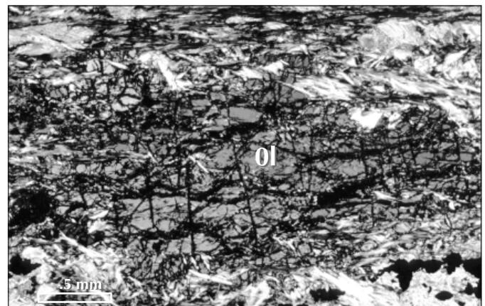
**Figure 5.** Enlarged view of the lower right section of Figure 4 showing the web-like alteration of olivine. Scale bar: 0.5 mm. XPL.
