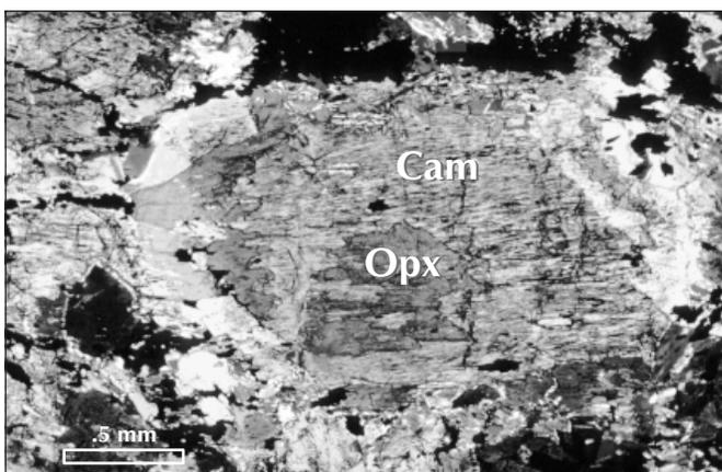
**Figure 9.** Photomicrograph of gabbronorite. The original orthopyroxene (Opx) is almost completely replaced by clinoamphibole (Cam) and only preserved as a relic in the centre of the crystal. Scale bar: 0.5 mm. XPL.
